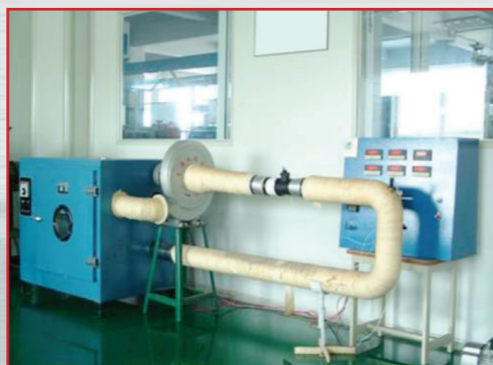
Test of the MAF at high temperatures of 120°C
