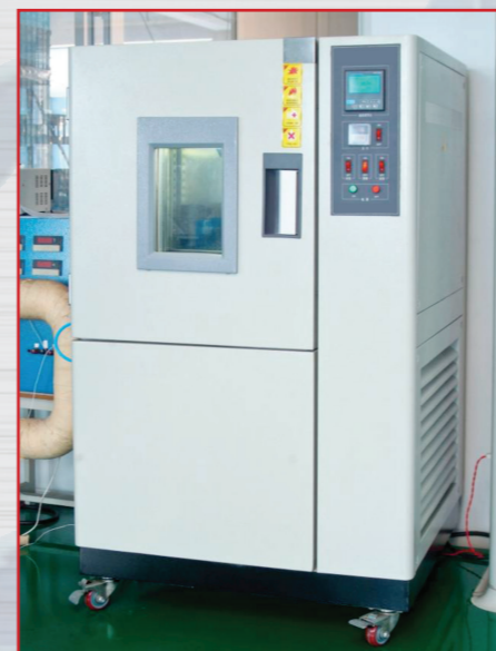
Changing temperatures from -40°C to 120°C
