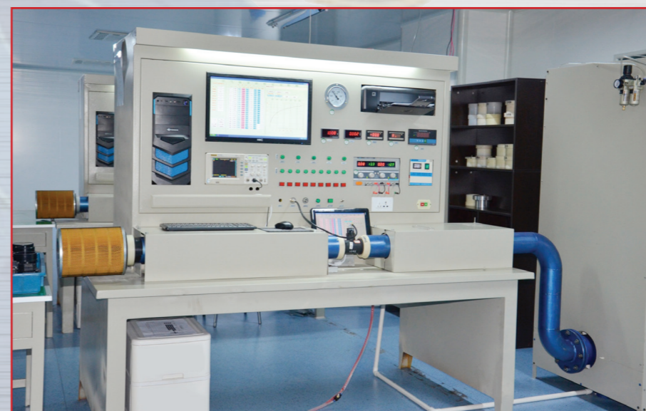
Final control Every MAF is finally calibrated
