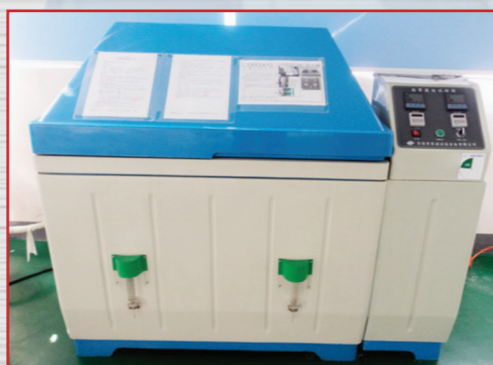
Test of susceptibility to corrosion 35+/-2°C – saltwater 5%, test period 96 hours
