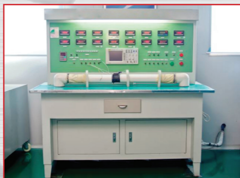
Test of the MAF at low temperatures of -15°C
